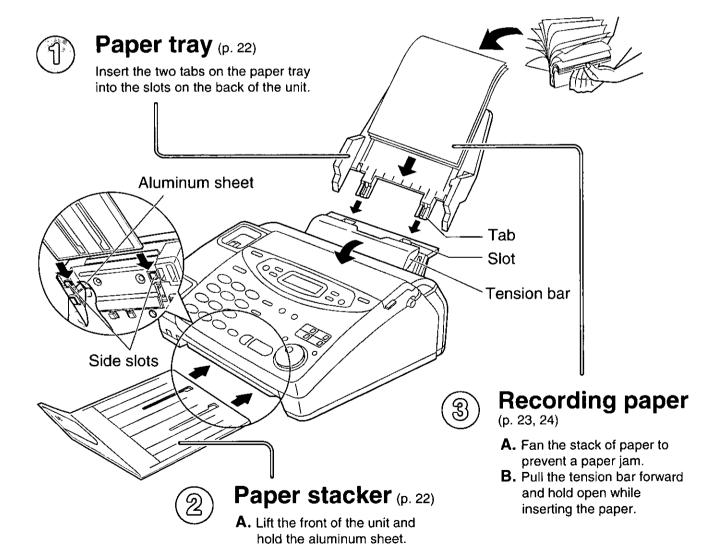
**B.** Insert the paper stacker into the side slots.
